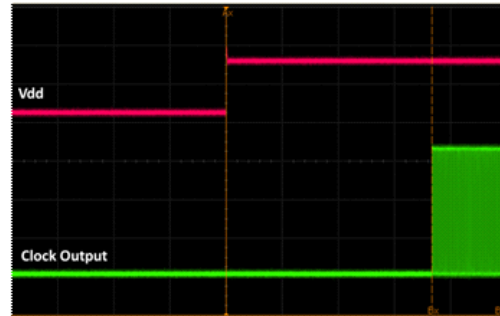
Figure 17. Startup Waveform vs. Vdd
